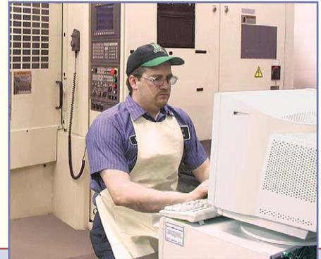
Shop floor in-process inspection is standard procedure. Our operators are trained and equipped with networked PCs on the shop floor to monitor the manufacturing process. We continually enter dimensional data and perform statistical evaluations to ensure our machining processes are producing parts within acceptable tolerance limits. Holding CPK's of 2.00 or greater on tolerances as tight as  $\pm .0002$  is common with our people and equipment.
