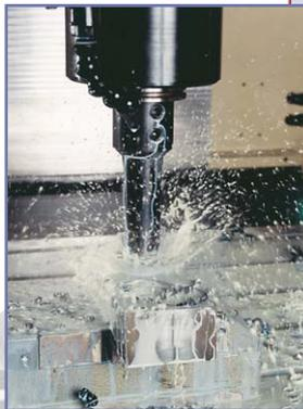
*Coolant through the spindle helps us drill holes faster and extends the life of our drills. According to Steve Swihart, "I recently inspected a \$250 drill that had drilled 15,000 holes... and it still looked new!"*
