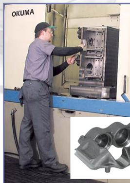
*This powerful Okuma machining center is not only able to take mega cuts in hardened steel, it can hold tolerances as tight as  $\pm .0002$ " to a CPK as high as 2.5.*
