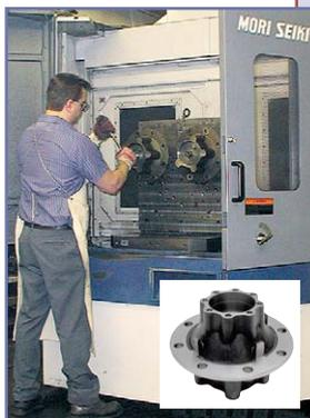
*Dual pallets and 60 tool positions are combined with 2 second tool changes and 1260 ipm traverse rates to give customers timely delivery at competitive prices. This Mori Seiki horizontal mill also excels at producing close, repeatable accuracy... it eats up high volume, tight tolerance jobs!*
