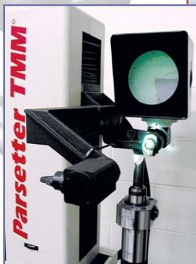
*Our Parlec Tool Presetter enables us to set our milling and boring tools "off-line" to tight tolerances. This dramatically reduces job setup time. And it helps make the first piece a good piece, which avoids scrapping your valuable workpieces.*
