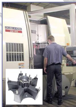
*Our twin spindle Okuma & Howa vertical lathes allow us to quickly and accurately turn out production for companies that require large turned parts. We have experienced CPK values as high as 2.5 on tolerances as tight as  $\pm .0015$ ".*
