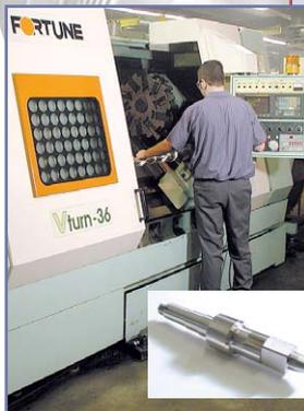
*Our family of horizontal lathes are accurate producers. This machine holds bearing journals to  $\pm .0002$ ", which enables our customer to save money in grinding operations.*
