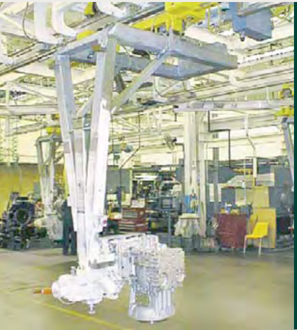
◀ Rugged transmission carriers provide complete access to workpieces
