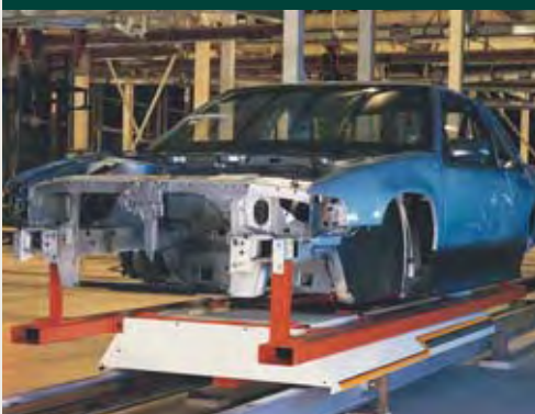
◀ Floor-mounted body assembly system
