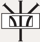
3-Way Switch Point
